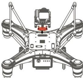
2. Plug the gimbal connector into the drone's gimbal port and screw it in place with a screwdriver.
