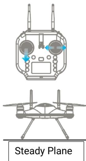
1. Place the drone on a level surface, power on the remote controller, then the drone. Wait for the aircraft to connect to the remote controller.
